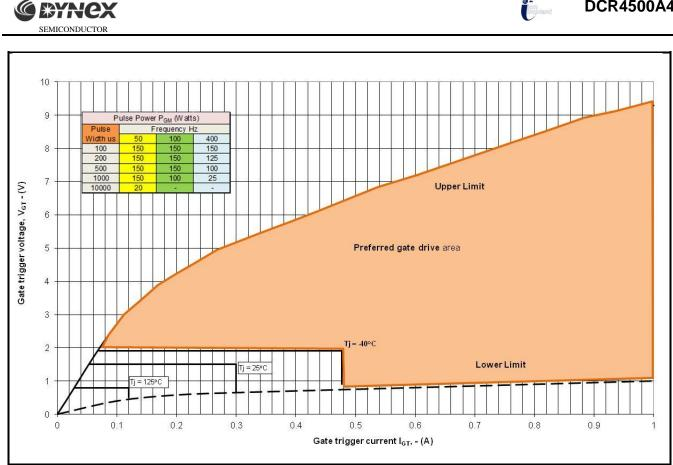
**Fig14 Gate Characteristics**
