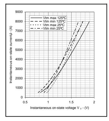
Fig.2 Maximum & minimum on-state characteristics
