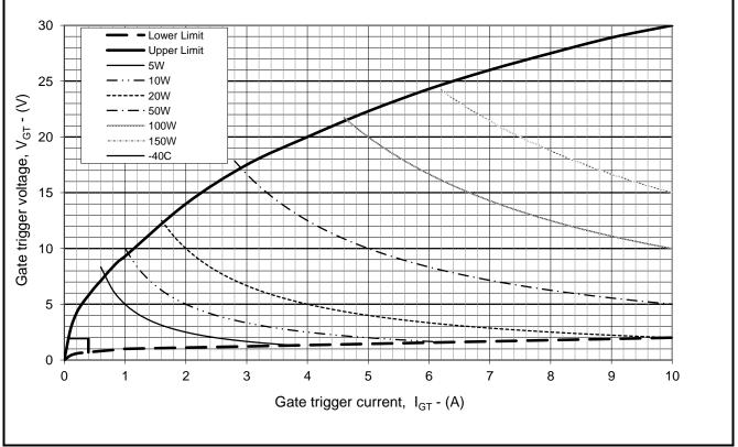
Fig. 15 Gate characteristics
